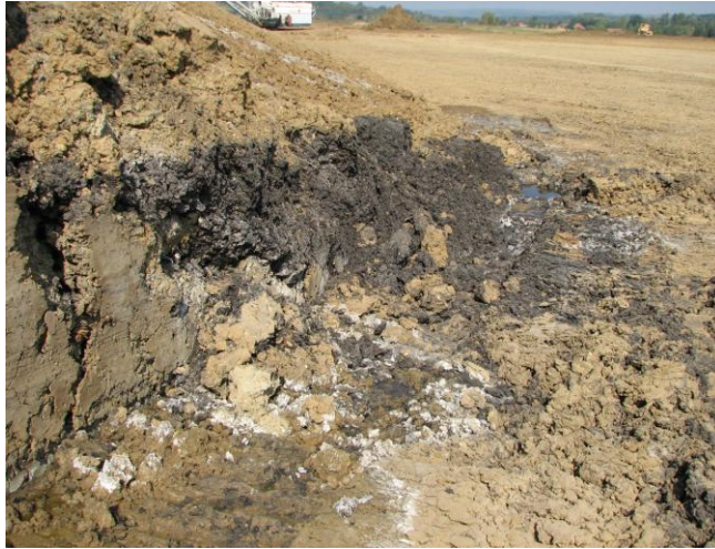
Figure 2. Mixed overburden layers on the final slope at the barren soil deposit 'Tamnava istočno polje'
