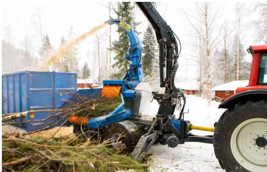
Figure 2: The Brooks mobile machine for wood chips (605PT Trailer)
