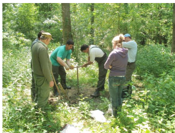
Figure. 3. Taking of samples with hand sonda. Srem, spring 2011.
