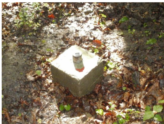
Figure 2. Piersometer station for water levels observation
