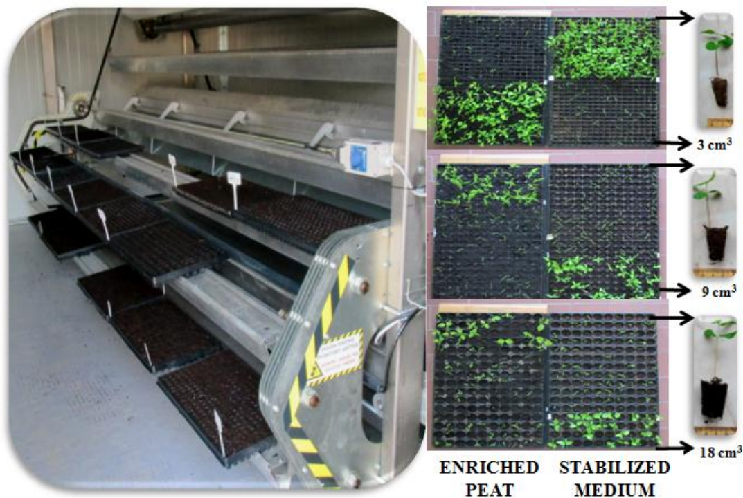
Photo 1. The prototype unit, the three mini-plug sizes (3-, 9-, and 18 cm 3 ) and the two soil substrates (enriched peat and stabilized medium).
