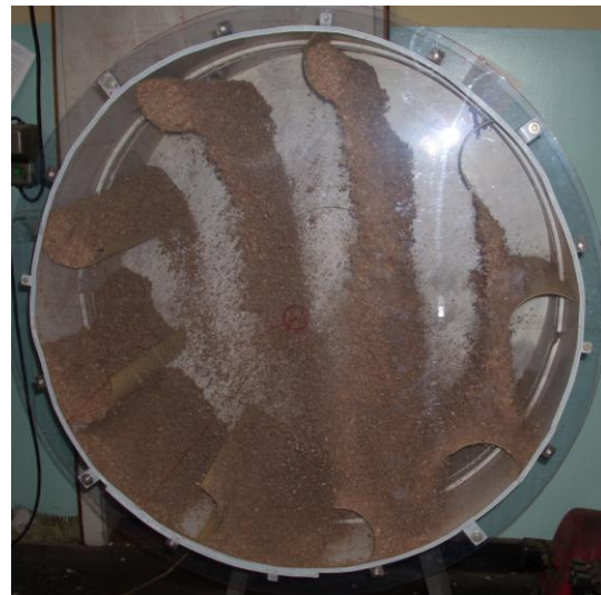
Figure 5: The model of drying chamber with flights
