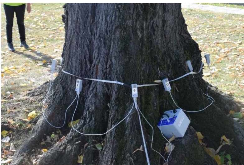
Figure 6. Arbotom sensors at height of 40cm with data receiver
